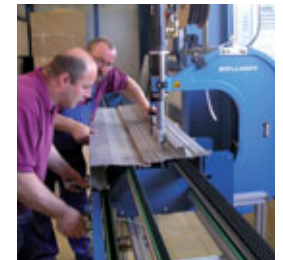
Production of air ducting segments with manually controlled components and integrated setting tool.
